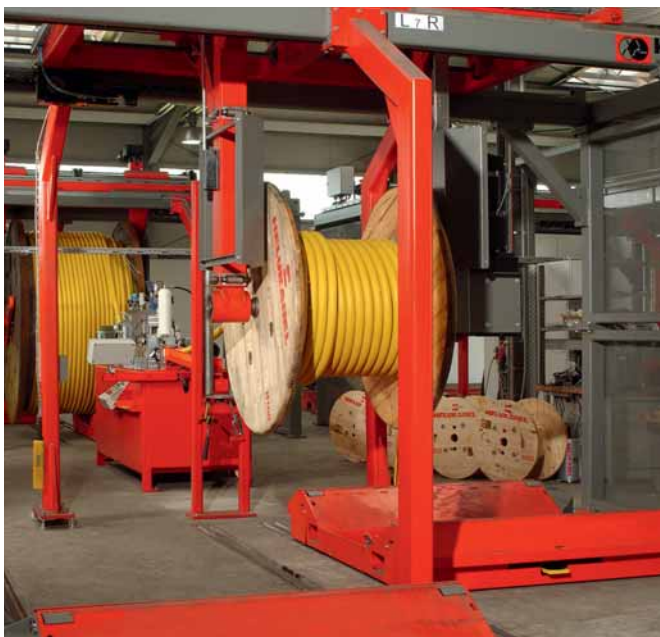
Heavy-load, cable-cutting facility
