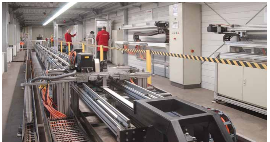
Drag chain test system
